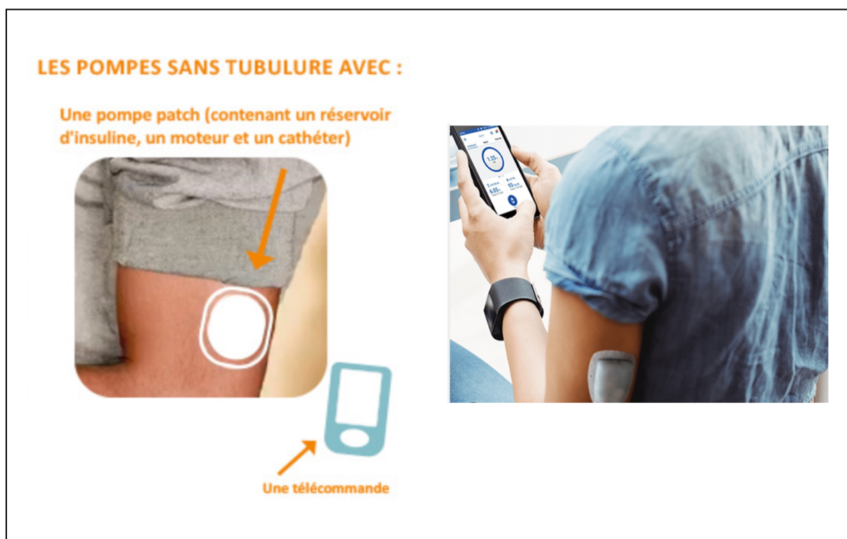
Figure 84 : Composants des pompes patch. [88]
