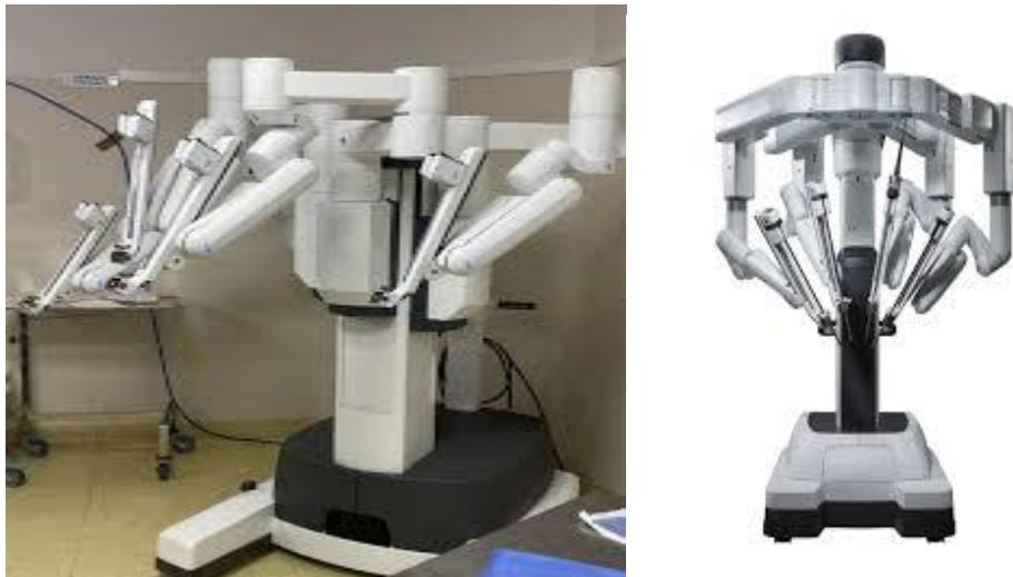
**Figure 65: Robot chirurgical Da Vinci 3 bras [51].**
