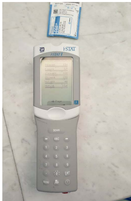
Figure 159: An example of POCT device available in our hospital: ABBOTT I-STAT. Measured parameters: Blood gas, electrolytes, hematocrit, glucose, lactate, creatinine, urea, cardiac biomarkers (Troponin I, BNP, and CK-MB), ionized calcium, coagulation (ACT and PT/INR) with 18 cartridges according to tests performed, 1 cartridge = 1 patient with Integrated quality control.
